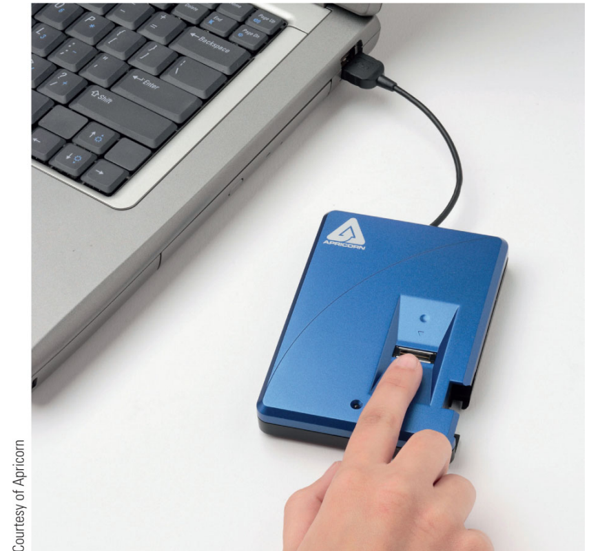
FIGURE 3-3 Encrypted hard drives. The data stored on this external hard drive is protected by a fingerprint scanner.
